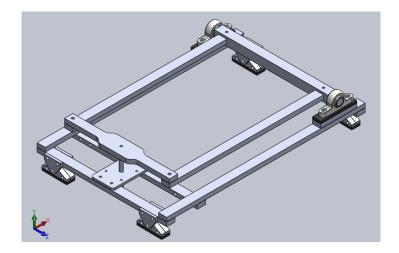
Install 2.5 kg masses at the four pendulum mounting points on the leveling system longitudinal struts (p/n-LSLS1) indicated below to simulate maximum loading of the test stand pendulum assembly
