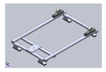
Mount NEMA 23 stepper motor with threaded pushrod onto the leveling system stepper motor mount, indicated in red, (p/n-SMM1) of the chamber interface
